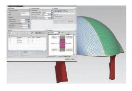
NX Laminate Composites NX Laminate Composites is a modular NX simulation toolset for laminate composite structures. Easy-to-use ply and laminate definition tools enable you to quickly create finite element models representing the laminate composite design. NX 7.5 improvements for Laminate Composites include enhanced modeling, import, export, postprocessing and journaling capabilities.
